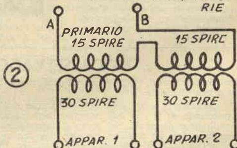
FINO A 4 APPARECCHI POSSONO FAR CAPO AD UN'ANTENNA CONICA USANDO QUESTI CIRCUITI IN TANDEM
